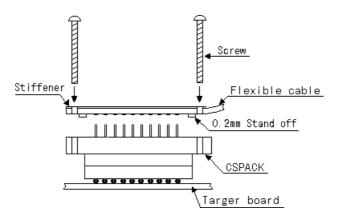
Fig. 4 Explosion view of ICE cable connection
