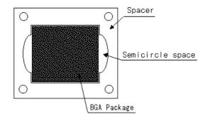
Fig. 2 Spacer and BGA package
