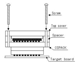
Fig. 3 Installing BGA package
