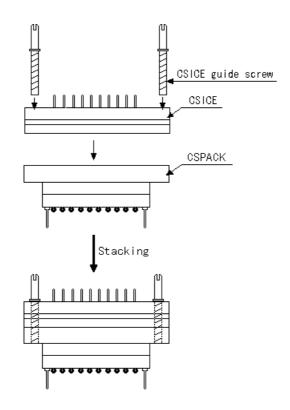
Fig. 5 CSICE stacking on CSPACK
