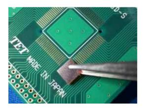
[3] When attaching, take care to align the stickers accurately with the foot pattern lines at each corner.
