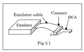
A polarity key prevents the user to plug the emulator cable and the SICA together in the wrong direction as shown in Fig 3.2
