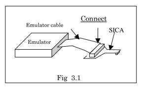
A polarity key prevents the user to plug the emulator cable and the SICA together in the wrong direction as shown in Fig 3.2. Check the key's position before assembling the header and the socket.
