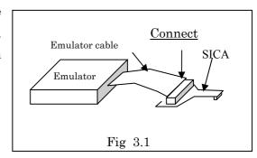
A polarity key prevents the user to plug the emulator cable and the SICA together in the wrong direction as shown in Fig 3.2. Check the key's porision before assembling the header and the socket.
