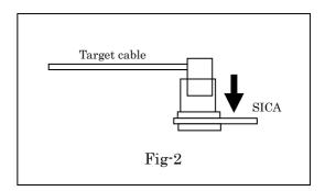
2) Connect the SICA38B40D-GG61 to the SICA2P40S socket on the target circuit board(see Figure 3). The connector design makes it impossible to connect the cable the wrong way around.
