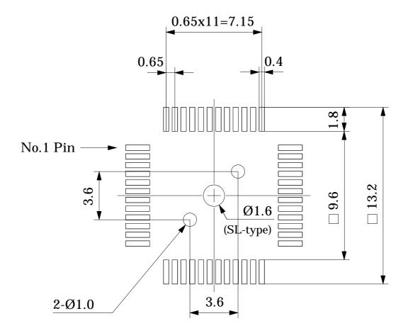
\* Recommended foot pattern shown on left is for NQPACK soldering. But please refer to IC package foot pattern recommended by IC manufacturer also, when the package is soldered on the same foot pattern.
