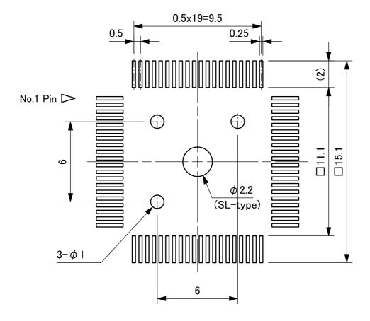
\* Recommended foot pattern shown on left is for NQPACK soldering.
