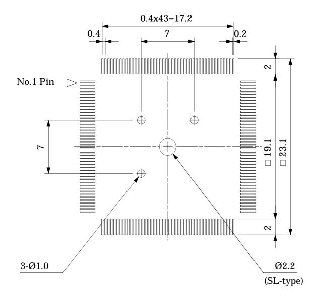
\* Recommended foot pattern shown on left is for NQPACK soldering. But please refer to IC package foot pattern recommended by IC manufacturer also, when the package is soldered on the same foot pattern.
