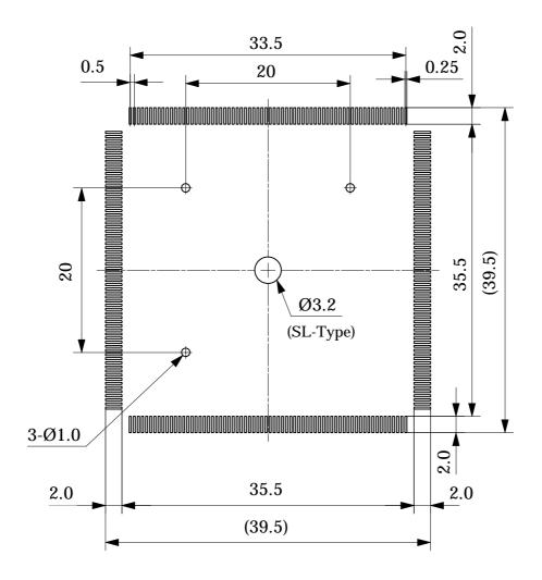
\* Recommended foot pattern shown on left is for NQPACK soldering. But please refer to IC package foot pattern recommended by IC manufacturer also, when the package is soldered on the same foot pattern.
