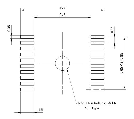
\* Recommended foot pattern shown above is for NSPACK soldering. But please refer to IC package foot pattern recommended by IC manufacturer also, when the package is soldered on the same foot pattern.
